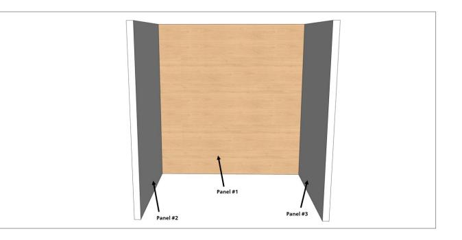
Place first spine panel, and ensure it is level. Use levelers to adjust if needed.
