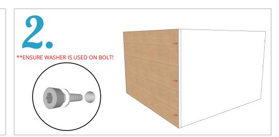
Line up spine and side panels #2 & #3 with holes to create 90 degree corner, and start all 3 bolts by hand until threads are engaged. Once engaged, tighten with cordless. Once complete, fasten the bolts tight and ensure both panels are level. Use levelers to adjust.
